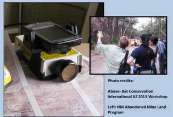
Figure 1. AnaBat SD CF Acoustic Bat Detector used to record bat calls.
