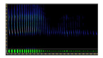
The gain setting on a detector allows users to "amplify" (e.g., strengthen, or make louder) a weak signal.
