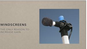
It's no coincidence that the only <u>bat</u> detectors with adjustable gains are the only detectors that offer a "windscreen." They are also the only detectors that began their lives as "acoustic" recorders, not "ultrasonic" recorders. Sound recording rules change for ultrasonic frequencies.
